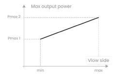
The maximum power the DCDC converter can provide is related to Vlow side range according to the chart beside.
